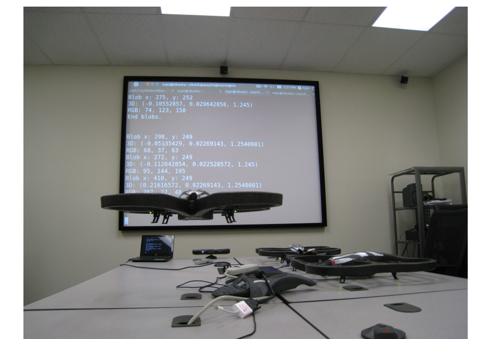
Vision-based localization experiment (utilizing Kinect 3D camera)
