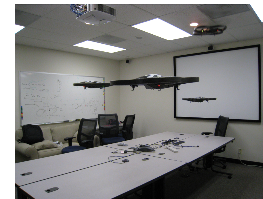
Four quadricopters controlled by the cyber-application framework
